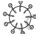
(c) Grease droplet surrounded by stearate ions (micelle formed)
