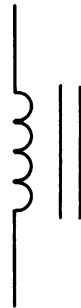
Fig. 4-16 The symbol for a coil with a core made of sheet iron.
