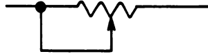
Fig. 2-18 A three-lead rheostat can easily be made to simulate a two-lead rheostat.
