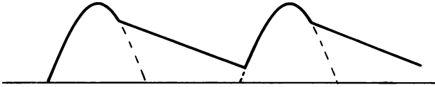
Fig. 5-16 Filtering the pulsating output of a diode rectifier gives a closer approximation of a dc voltage.
