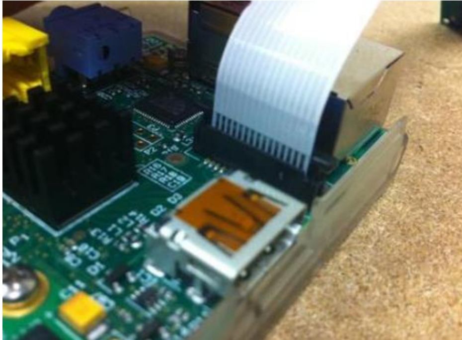
Figure 3.4: Interfacing camera module to raspberry Pi
