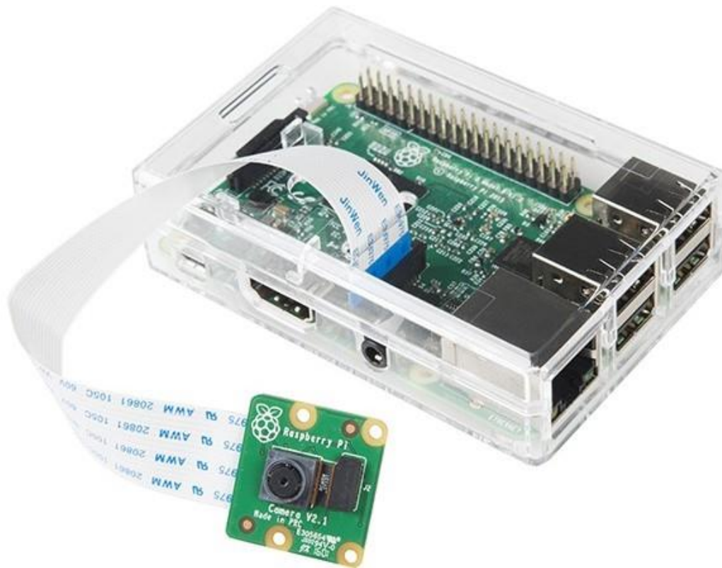
Figure 3.1: Raspberry pi 3 interface with camera module
