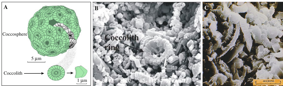
Fig. 5.10 (a) Skeletal structure of coccospheres and coccoliths. In this example the spheroidal coccosphere is composed of many round calcareous plates (coccoliths) which consist of tiny, platy calcite crystals stacked in an imbricate pattern. Modified from Hjuler (2001). (b) SEM picture of Liège chalk consisting
