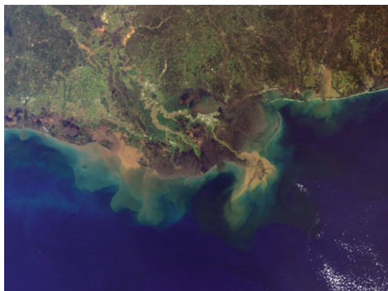
Fig. 6.1 Satellite photograph showing the distribution of clay outside the Mississippi delta. The limited extent of the delta mud is due to flocculation of the clay particles when freshwater is mixed with ocean water
