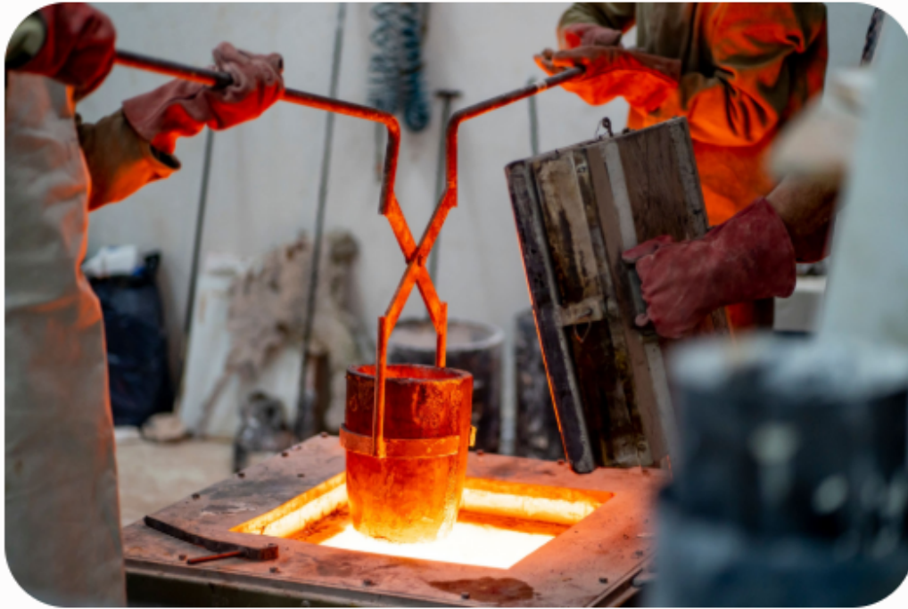
Lifting a heated crucible using purpose-fit tongs. Source: Westend61 / Getty Images
