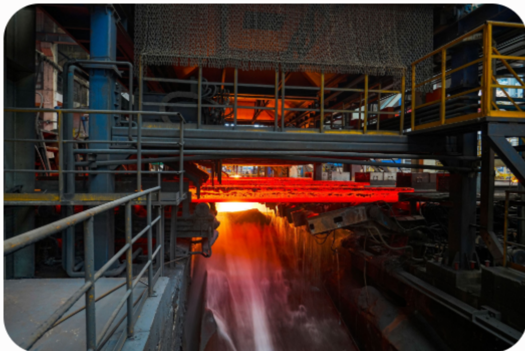
Hot steel billet traveling through rolling mill stands. Source: songqiuju / Getty Images
