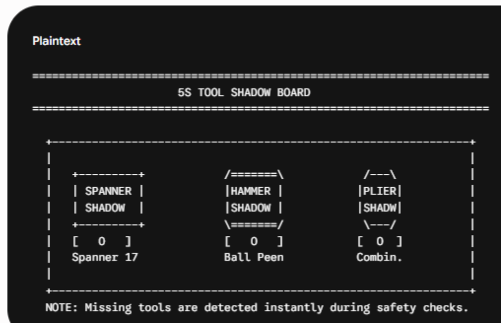
Sketch 1: Seiton (Set in Order) Tool Shadow Board
