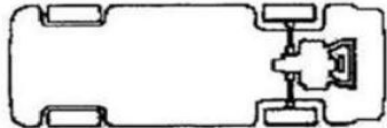
Rear-engine and rear-wheel drive c.coomarasamy
