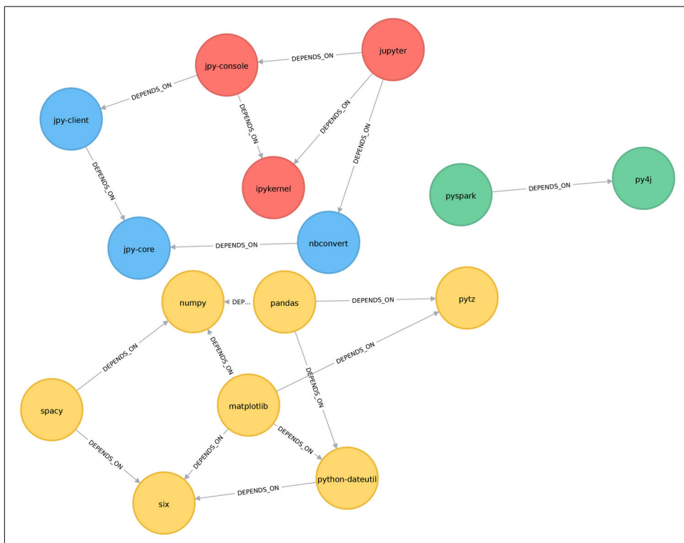
Figure 6-10. Clusters found by the Label Propagation algorithm, when ignoring relationship direction
